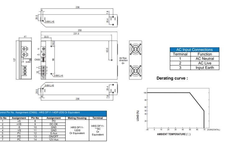
\*The power supply will have no output if the shorting connector CN50 is not assembled. It contains 3 shorting wires: one is from on/off (pin13) to 12V-Aux (pin14), 2nd is from PC (pin7) to PO (pin8) and the 3rd is from PV (pin5) to PS (pin6)
