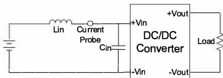
**Output Ripple & Noise Measurement Test**
