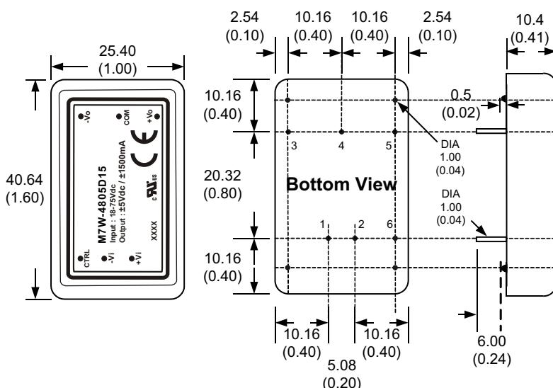
All dimensions are typical in millimeters ( inches ).
