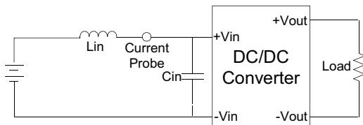
**Output Ripple & Noise Measurement Test**
