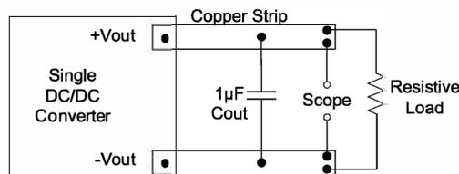
**Input Reflected Ripple Current Test Step**
